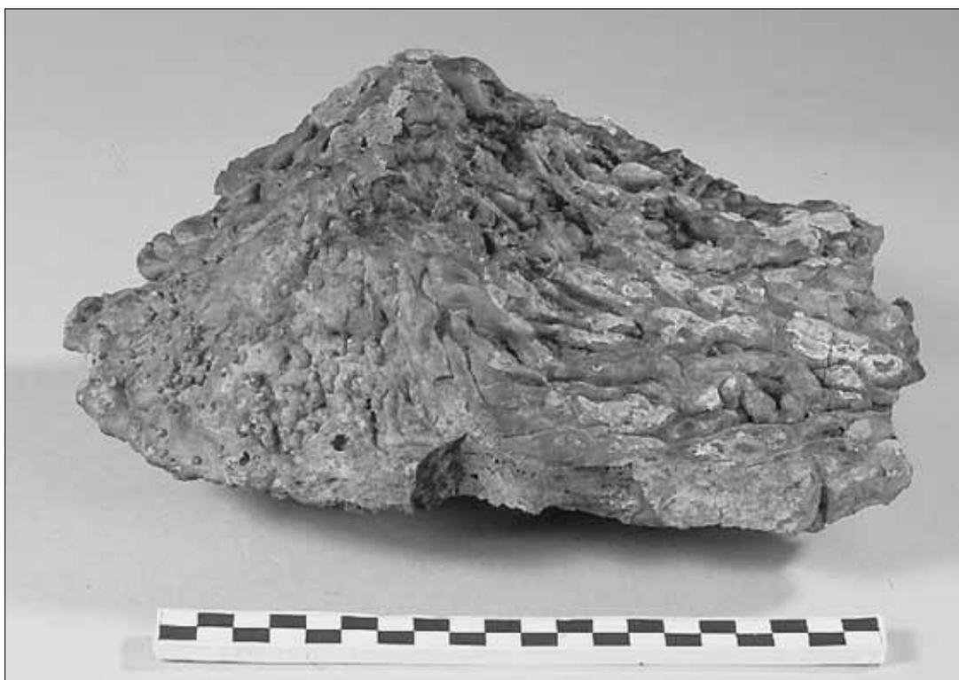
Fig. 18 Cone-shaped tap slag (photo by: N. Sautner)
