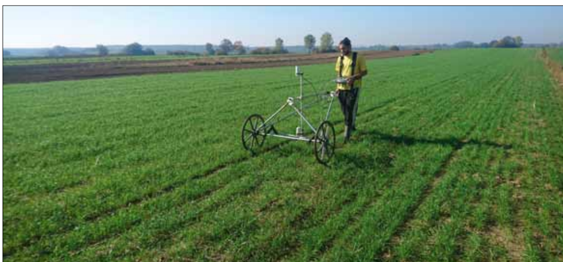
Fig. 2 Magnetometer Geometrics G-858 in gradient mode fixed on survey cart for constant position of sensors above ground during survey at archaeological site of Velike Hlebine (foto by: B. Mušič)
