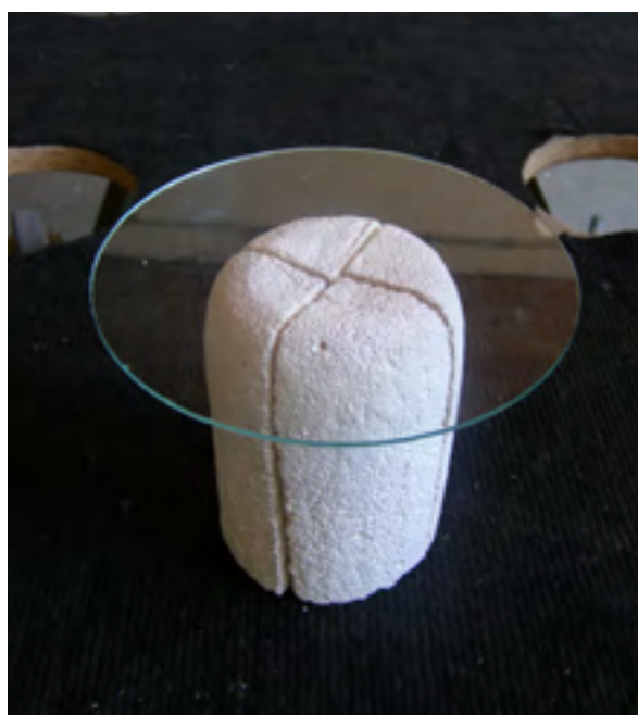
Sl.12 Kalup za fuziju stakla (snimio: Š. Perović 2012) Fig.12 Mold for glass fusing (photo: Š. Perović 2012)
