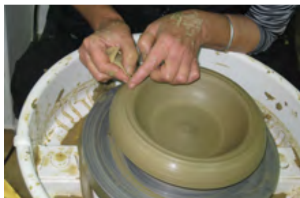
Sl. 8 Izrada uvučenog dijela oboda tarionika Fig. 8 Making the indented part of the mortarium's rim
