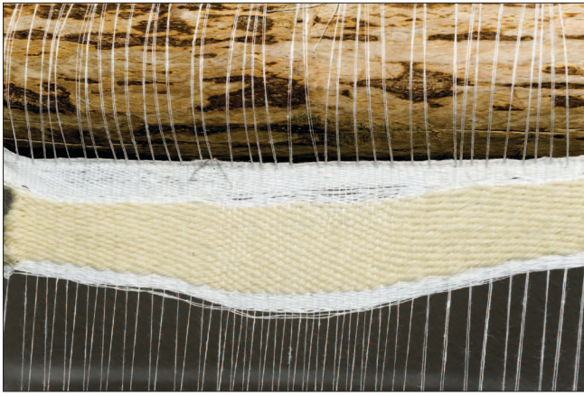
Sl. 13 Gušći, srednji dio tkanine zakrivljen prema dolje Fig. 13 Curving down of the middle denser part of the textile
