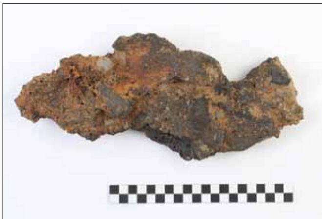
Fig. 9 Fragment of slag from inside furnace (photo by: H. Jambrek)
