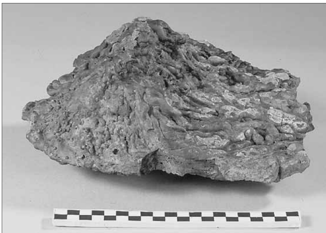
Fig. 18 Cone-shaped tap slag (photo by: N. Sautner)
