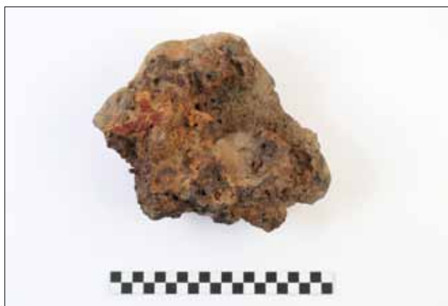
Fig. 12 The fragment of furnace wall with attached slag and solid particles of iron ore from the Okuje site (photo by: H. Jambrek)
