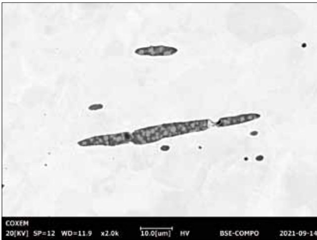
Fig. 8a Typical small elongated two-phase slag inclusion with fragmented fayalite laths (light grey) in glassy matrix (dark grey) (SEM-BSE photo: D. Doračić)
