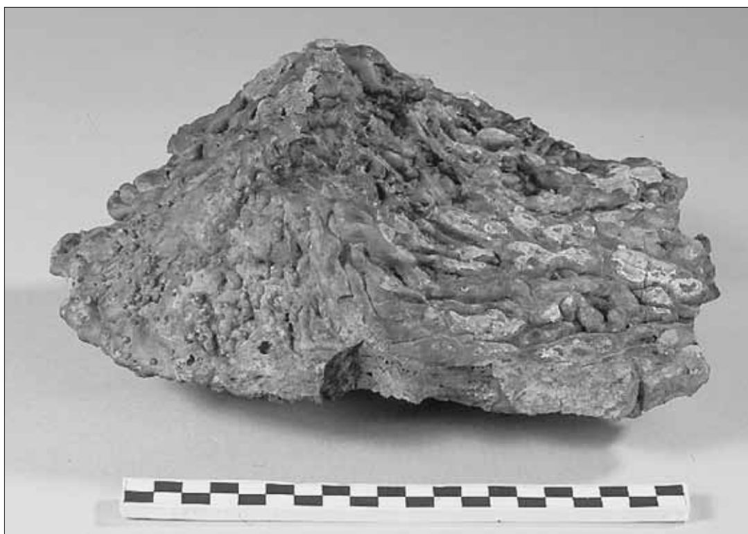
Fig. 18 Cone-shaped tap slag (photo by: N. Sautner)
