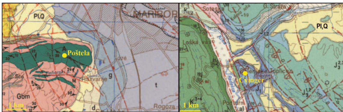
Fig. 2 Geological maps of the researched areas. Left: Poštela: A – amphibolite; Gmb – muscovite-biotite gneiss; PI, Q – conglomerates, sand, sandy clay, clayey gravel; g – sandy clay; t – fluvial terraces. Right: Cvinger: J 1,2 – light grey stratified limestone with oolites (upper lias, dogger); PI, Q – brown loamy weathered sediment and terra rossa (source: Osnovna geološka karta Slovenije / The basic geological map of Slovenia, excerpts of pages Maribor (left) and Novo Mesto (right), link: http://biotit.geo-zs.si/ogk100/ , modified by B. Horn)
