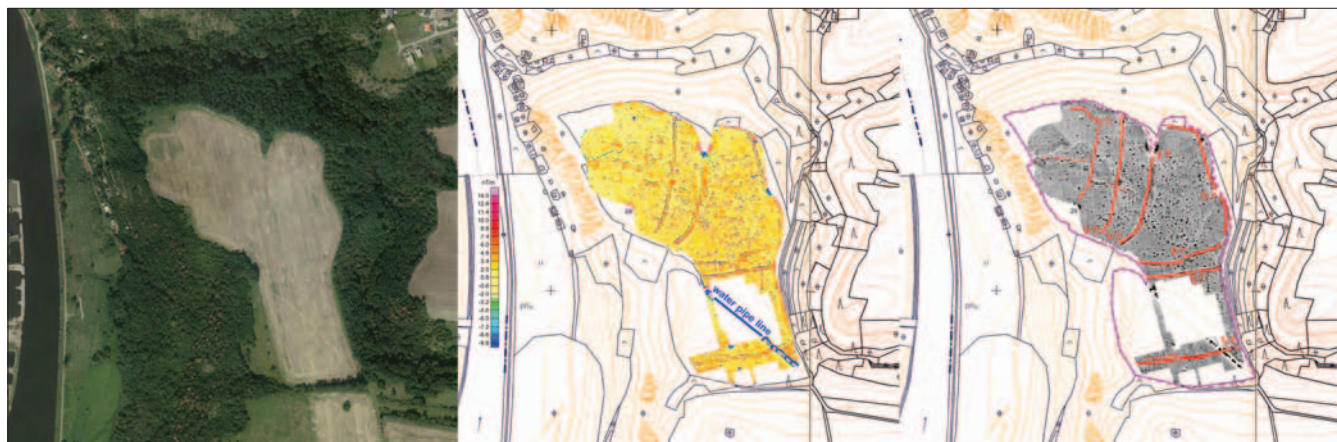
Fig. 1 Zlončice, district Mělník. Comparison of aerial photograph and result of magnetometer survey with interpretation of ditch fortifications and entrances on base map (source: www.kontaminace.cenia.cz ; surveyed area: approx. 9.5 ha; survey: Křivánek, 2008–2010)
