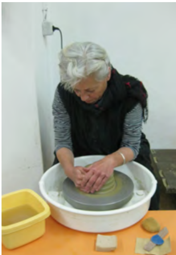
Sl. 1 Početak izrade dna - centriranje Fig. 1 The beginning of base production - centering
