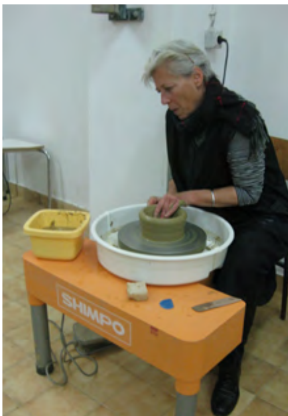
Sl. 2 Izrada stjenke posude (otvaranje) Fig. 2 Making the vessel walls (opening)
