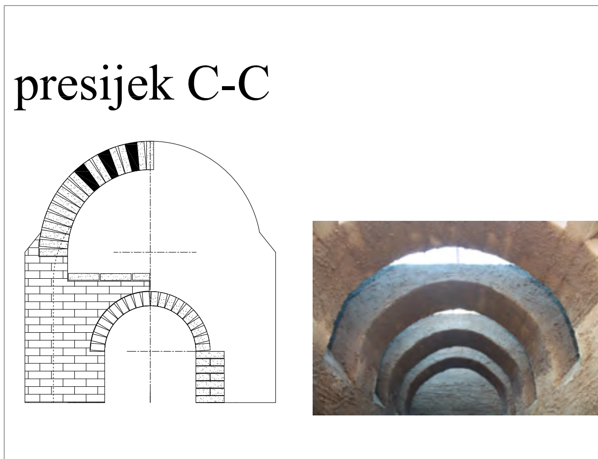
Sl. 13 Lukovi mostova koji razdvajaju dimnu komoru od radne komore Fig. 13 Arches of the bridges which separate the smoke chamber from the working chamber
