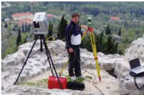
Fig. 1 3D laser scanning fieldwork Sl. 1 Terenski rad na 3D laserskom skeniranju
