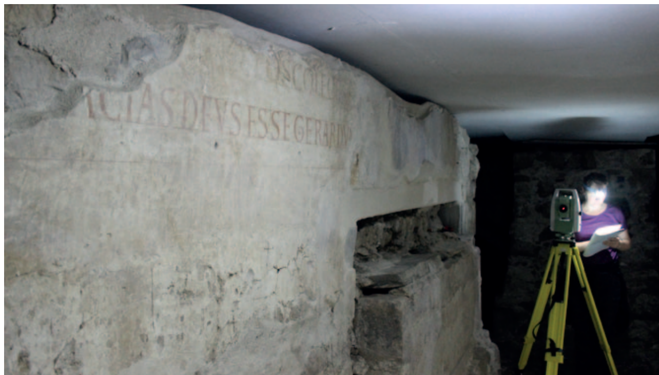
Sl. 2. Pogled na vanjski perimetralni zid prve crkve s monumentalnim grobnicama u tijeku snimanja totalnom stanicom (snimila: I. Ožanić Roguljić) Fig. 2. View of the outer perimeter wall of the first church with the monumental tombs during total station recording (photo: I. Ožanić Roguljić)
