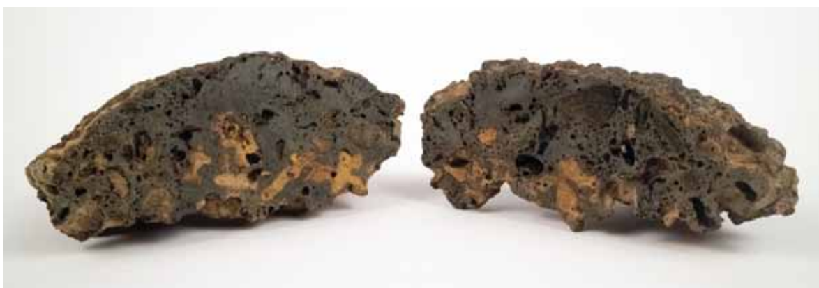
Fig. 8 A post-reduction slag with a piece of charcoal in the slag mass (photo by: M. Gregl)
