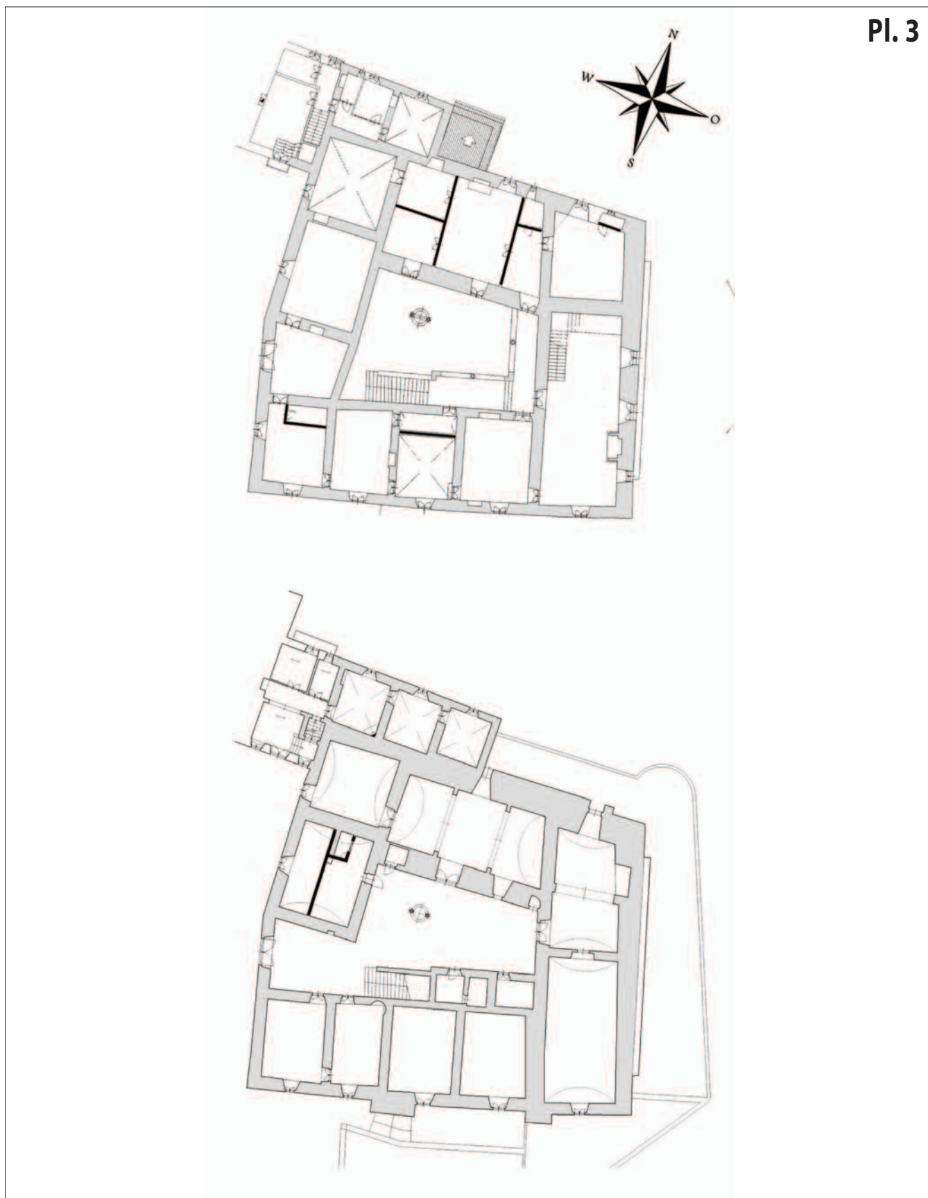
Pl. 3 The Cantelmos Castle of Bussi – maps of the ground floor and first floor: partition of the mansion into several residences (drawing by: C. Mazzanti 2015)
