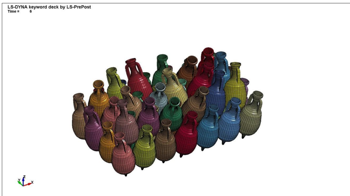
Figure 1 – Finite element model of an amphorae group
