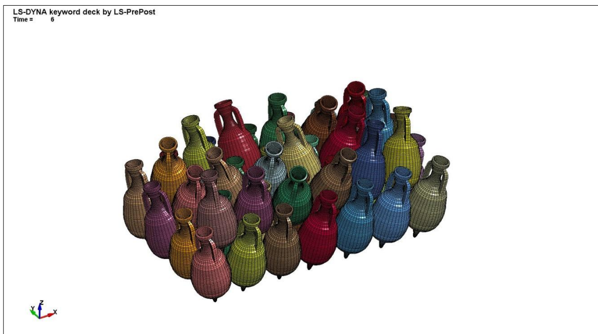
Figure 1 – Finite element model of an amphorae group
