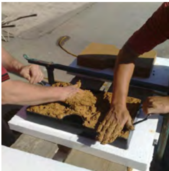
Sl. 7 Ručna izrada ploča rešetke u kalupu (foto: Mužek Kaminko d.o.o.) Fig. 7 Making of slabs for the grid by hand using the mold (photo: Mužek Kaminko d.o.o.)
