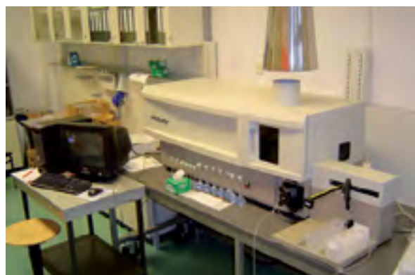
Sl. 4 Instrument: ICP-AES, Teledyne Leeman PRODIGY, USA
