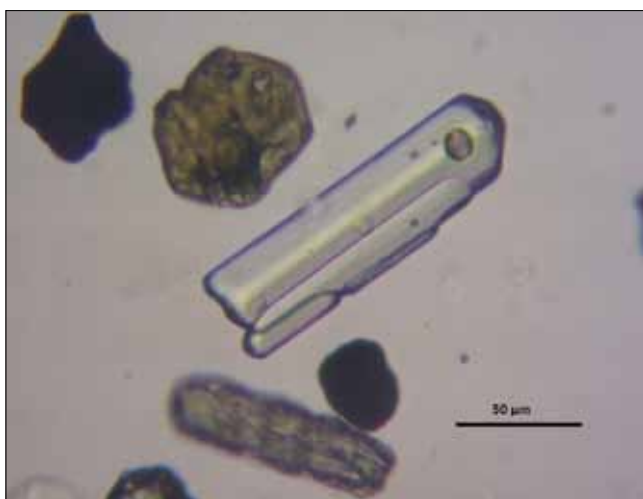
Sl. 5 i 6 Mikroskopski preparat s izdvojenim zrnima vulkanskog stakla iz sloja tefre veličine do 50 mikrona (DIV-2) – smeđa zrna s paralelnim crnim crtama (snimio: I. Razum) Fig. 5 and 6 Microscopic sample with grains of volcanic glass from the tephra layer up to 50 microns big (DIV-2) brown grains with parallel black lines (photo: I. Razum)
